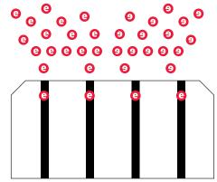
quality of the cell and the solder between them. Thus, the Hero series is made of the best "A" quality cell and 9 guidewires. Over the long years, it matters a lot if even 1 in 4 to 6 conductors detaches from the cell surface 4-6 conductors, a fault due to soldering or because the energy produced cannot pass a change in cold-heat can cause a serious through. In the case of 9 guide wires, this is not possible!
